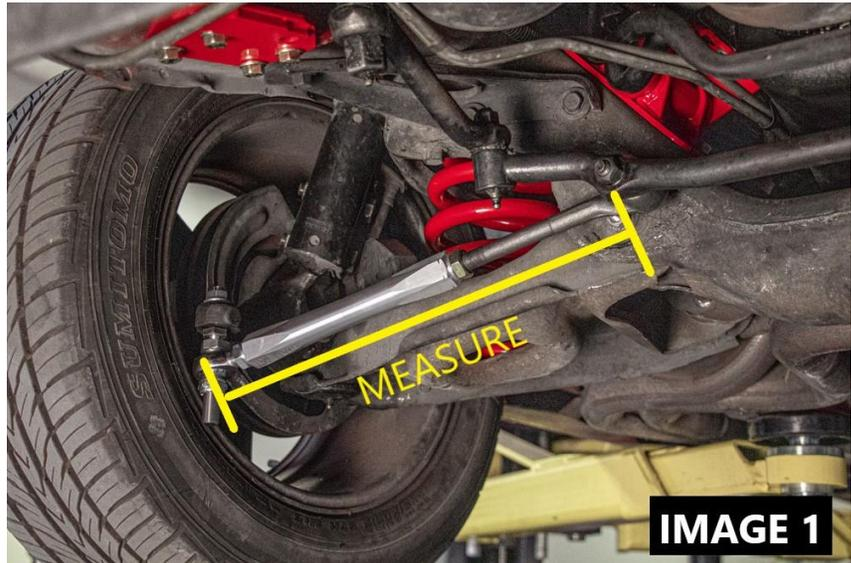
3. Measure the distance from the inner tie rod end to the outer tie rod end **IMAGE 1**
