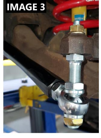
ADJUSTER. IF YOU HAVE MORE THAN 8 THREADS EXPOSED, YOU WILL NEED TO ADJUST THE LENGTH OF THE ALUMINUM ADJUSTER ON THE INNER TIE ROD.
