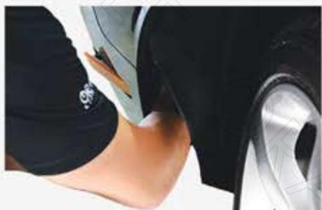
REACH INTO THE WHEEL WELL, SQUEEZE THE CLIPS ON THE BACK OF THE STOCK SIDEMARKER AND REMOVE IT
