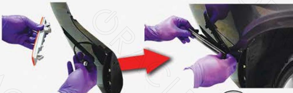
UNCLIP THE STOCK SIDEMARKER, AND THEN REPLACE IT WITH YOUR NEW ORACLE LED SIDEMARKER. PUSH YOUR WHEEL LINER INTO PLACE AND REPLACE YOUR RIVETS.
