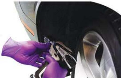
REMOVE THE THREE (3) RIVETS IN THE WHEEL WELL THEN PEEL THE WHEEL LINER BACK
