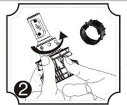
Install the collar into the headlight socket and twist into place.
