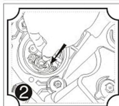
Align the collar of the bulb in the factory socket and use the metal clamp to lock it into place.
