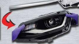
· Now place the housing back into place on the headlight & then reinstall the six T-25 screws back into the headlight
