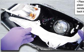
· Place the Diffuser back into place inside the headlight & then reinstall the four T-25 screws back into the Diffuser
