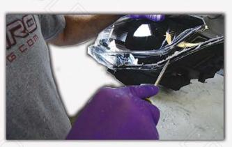
A) Start by using a flat-head screwdriver and apply pressure between the lens and housing. CAUTION! Headlight will be hot.
