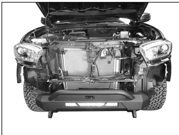
(Fig 3) Remove factory hardware along the ends, top and bottom to remove cover
