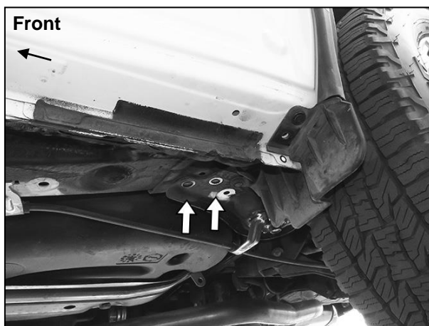
(Fig 15) Remove (2) factory hex bolts (arrows)
