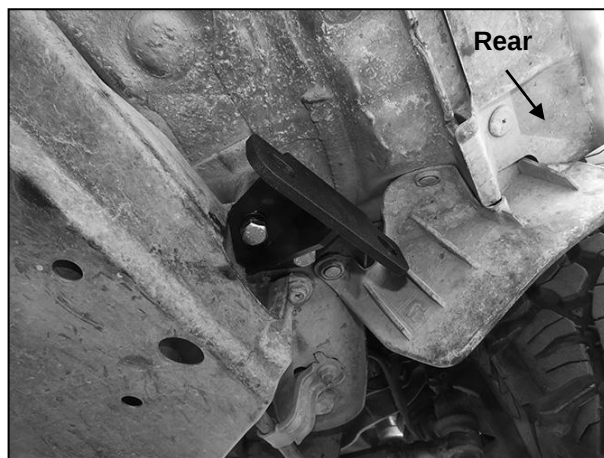
(Fig 9) Driver/left rear Bracket installed over aftermarket suspension lift spacer.
