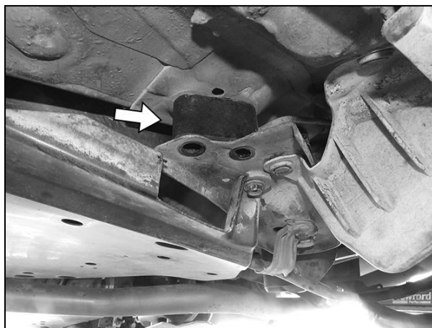
(Fig 7) Example of model with aftermarket suspension lift "spacer" (arrow)
