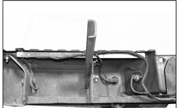
(Fig 6) Remove license plate lights, wiring harness and parking sensors from factory bumper as equipped
