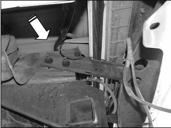
(Fig 1) Remove hex nuts from bumper brackets Unplug and move wiring harness away from bumper
