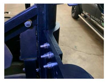
Install pods with four M6 cap head bolts using a 5mm Allen wrench and connect wiring
