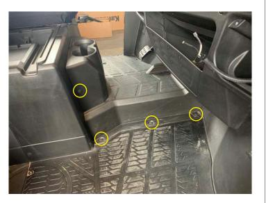
• Remove five push pins from the driver side center console
