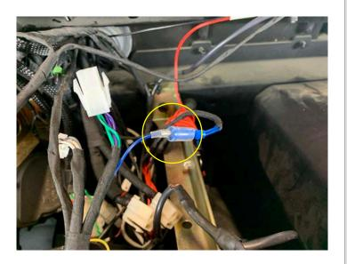
• Route the rear speakers and subwoofer extension harness from the middle of the dash out the grommet toward the front of the vehicle
