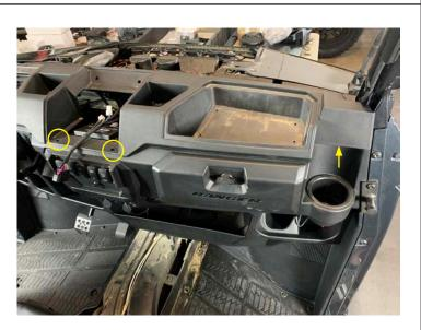
Install upper glove box with four T20 Torx screws
