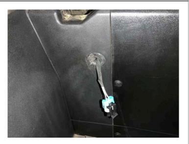
• If four-seat vehicle, connect extension harness to route rear speaker wires to the back of the vehicle if installing rear pods jump to that section
