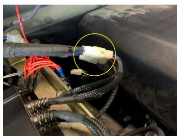
• Plug in the amplifier harness connectors to the amplifiers
