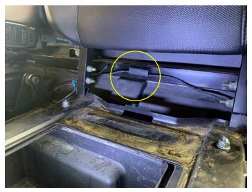
Route driver side green speakers wire-in channels toward driver door. Then route upward toward the ROPS (avoiding any moving objects), secure, and attach one adhesive channel on ROPS
