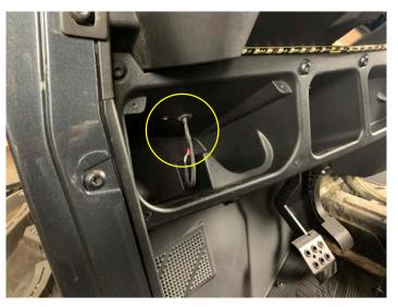
• Reaching from the top of the passenger side of the dash, pass the gray wires through the top of the pocket and insert the grommet
