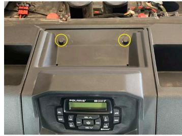
• Remove two push pins from center cup holder
