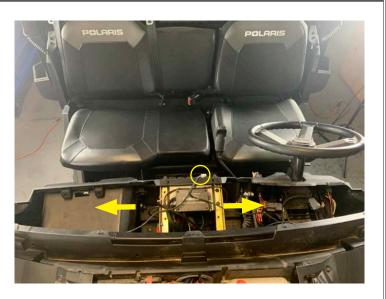
• Reaching from the top of the driver side of the dash, pass the white wires through the top of the pocket and insert the grommet
