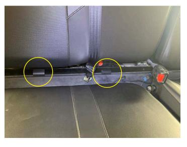
Route passenger side violet speakers wire-in channels toward passenger door, then route upward toward the ROPS (avoiding any moving objects), secure, and attach one adhesive channel on ROPS
