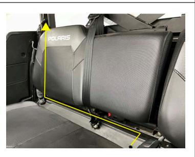
• Place one adhesive channel on driver side under seat on frame
