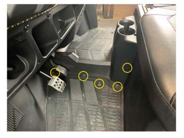
• Lift center console upward starting at cupholder and remove from vehicle
