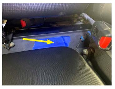
• Drill 1/2" hole and then pass rear speaker wire from battery compartment out to inside of passenger cabin
