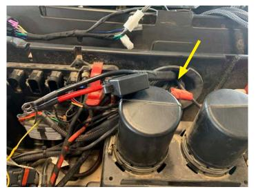
• Connect the power and ground wires by removing the 10mm nuts on the pulse junction block
