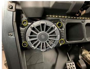
• Connect the speaker wires to the speaker and then install the speaker and grill assembly with four high-low torx screws and washers using a T25 Torx bit
