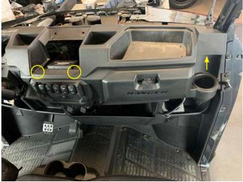
• Remove three push pins on the driver side dash
