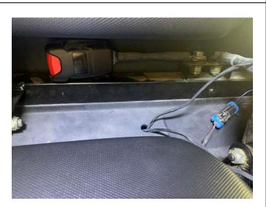
• Pass speaker wires through grommet and insert grommet into the drilled hole
