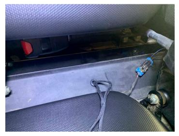
• Place two adhesive channels on passenger side under the seat on the metal frame
