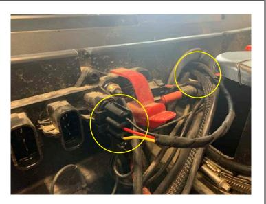
• Pass the amplifier power harness from the front of the vehicle into the cab through the grommet
