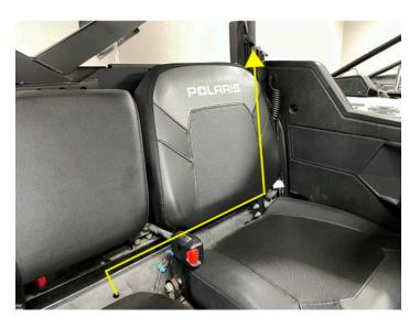
• Position bracket on the ROPS and secure with four M6 bolts with a 5mm Allen wrench and 13mm socket (same process on passenger and driver side)
