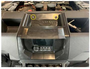
• Place center console in the vehicle sliding forward then down
