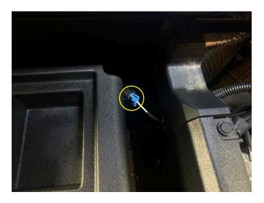
• Attach the left and right harness to bullet connectors in the center console
