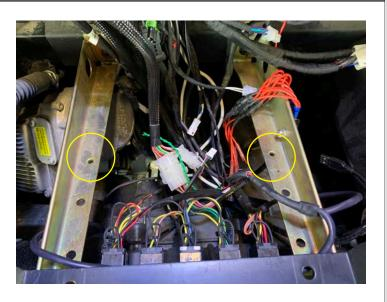
• Raise the plate and install two 10-32 x <sup>3</sup>/<sub>4</sub>" bolt and washer into amplifier plate
