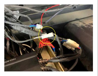
• Connect the speaker y-harness to the front and rear speaker harnesses
