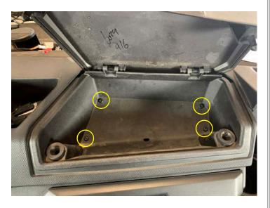
• Remove three push pins on the passenger side dash
