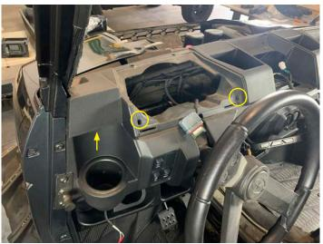
• Connect harness and place the instrument panel in location and then insert two push pins
