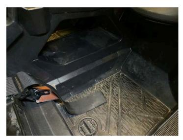
Install rear glove box in rear center console (Remember to connect wires to bottom 12-volt accessory port)
