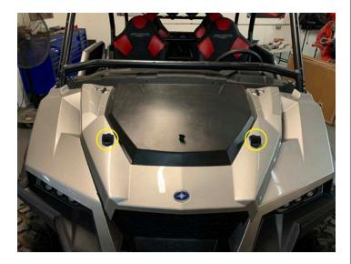
• Remove seven push clips from front of dash
