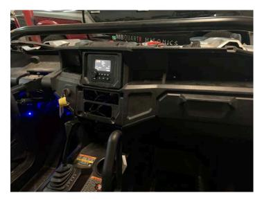
Install key switch and align to detent
