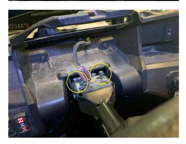
• Install two T40 bolts in center console
