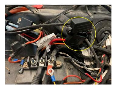
Remove Delphi connector at bullet and pass these wires along with the amplifier connector from hood area to the inside through the grommet
