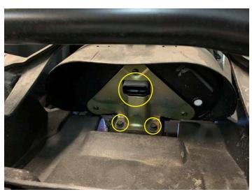
Disconnect the connectors from the back of the light and four wheel drive switches
