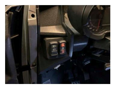
• Remove two T40 bolts from the instrument cluster pocket
