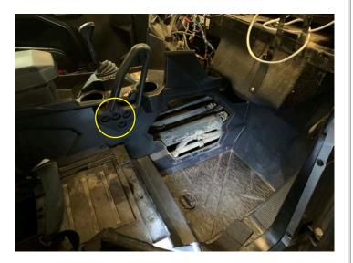
• Install center cover with two push pins
