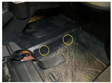
If two-seat skip ahead, If four- seat then install rear console and install six push pins on driver and passenger side
