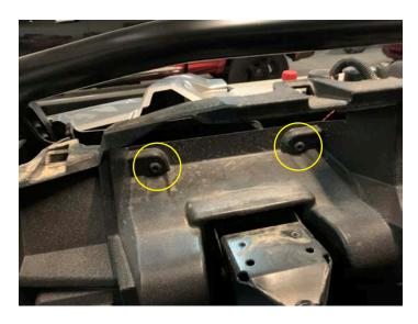
Carefully pull dash toward rear of vehicle by door opening on driver and passenger sides
