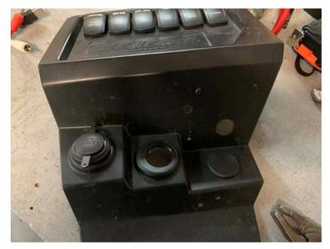
• Install the USB / AUX port in this hole (PASP-18)
