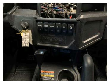
• Disconnect wires from back of 12-volt accessory port
