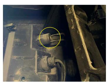
• Remove plastic nut from ignition switch and remove from dash
