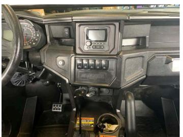
• Install top of dash, snapping eight push clips on front of dash
