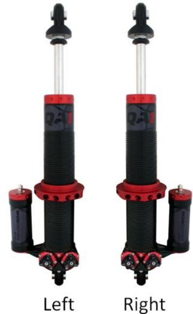
1. Before starting the installation, check the part number of the shock and the recommended ride height measurement in the chart below compared to the mount-to-mount dimension of the vehicle at ride height. If the shocks are mounted outside of the recommended ride height range, the shocks may be damaged in operation. The shock part number and serial number are etched on the Schrader valve end of the canister.
