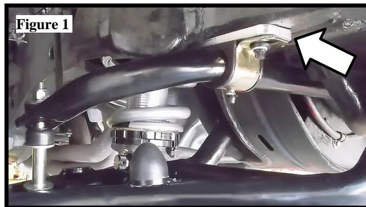
8. Compress the suspension by setting the vehicle on the ground before connecting the sway bar end links to the control arm. The new end link bushings having never been compressed can make the bolt appear to be too short. Further compression of the sway bar to control arm may be necessary to get the end link nut started.
