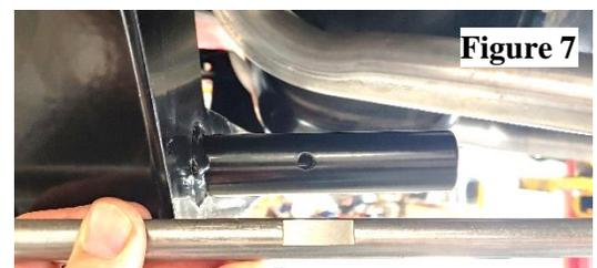
9. Center the pivot shaft in the cross-member by looking through the set screw hole of the crossmember and lining up the flat of the pivot shaft. **(Figure 8)** Install the set screw with blue Loctite and torque to 13 lb. ft.
