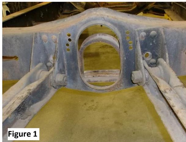
4. Unbolt the truck arm front attachment bolts. Lower the arms down and support with stands. **Caution:** Do not kink or allow the axle to pull on the brake hose.
