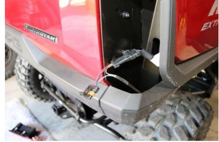
3. Unroll the long extension cable and plug it into the rear harness, run the cable along the frame to the battery compartment, remove the rocker panel and run the cable through the frame up to the control module. Lift up on the floor and feed the cable through the floor at the arrows.
