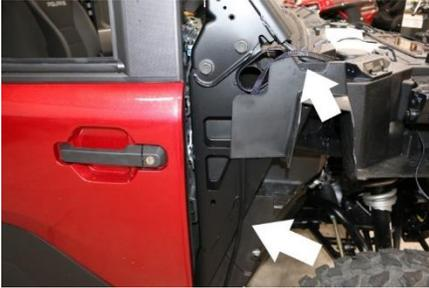
**WARNING! Verify that there is clearance where you want to mount the front LED lights before drilling the holes.**
