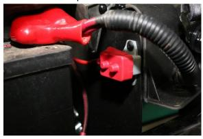
5. Attach the 18" long Red 8GA power wire from the Fuse Block over to the center post on the factory Busbar
