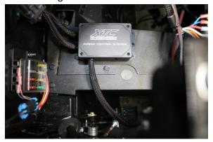
**3.** Mount the Fuse Box on the fire wall above the control box.
