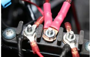
**6.** Attach the Long 6' 8GA wire to the Busbar and install Keps Nut, run cable down through center console to the Circuit Breakers Silver Screw terminal and attach. The 6" cable that is attached to the copper terminal now gets attached to the positive Battery Post.
