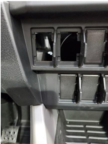
3. Remove the switch from the harness and from inside the dash run the 8-pin connector through the rectangle, plug the switch in to it and insert into dash. **NOTE:** On the new **XP PRO** the dash has an indent, to make the standard switch work in the opening it requires the use of 2 seals. They can be ordered if needed at [www.xtcpowerproducts.com](http://www.xtcpowerproducts.com)
