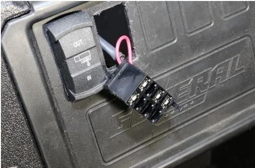
6. Plug the horn switch into the connector and install into the cutout
