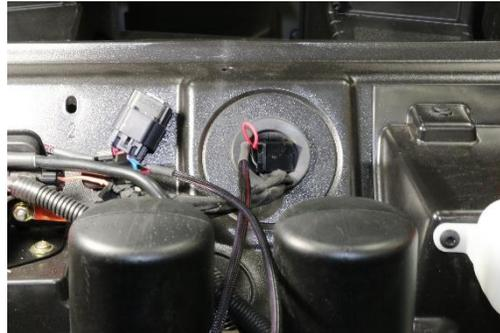
5. Cut out one of the switch mounts and run the 8-pin connector through the cutout
