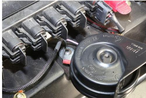
3. Mount the horn using the provided screw as shown above
