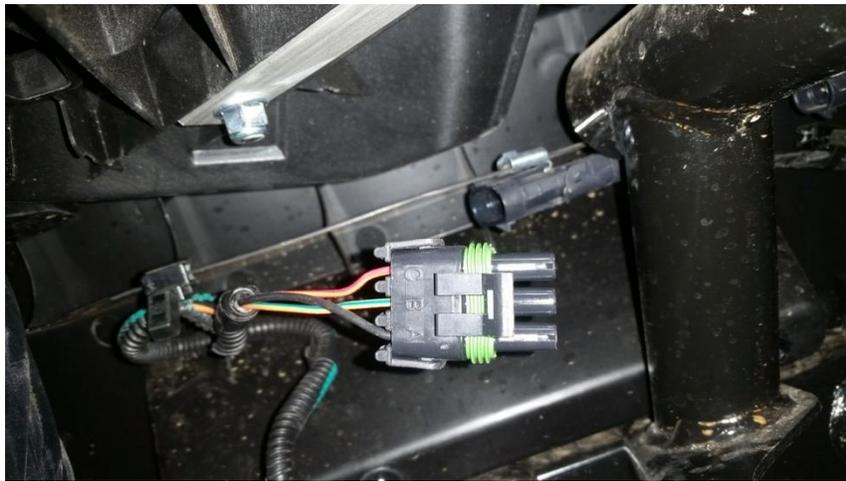
1. Unplug OEM light connector at either Side inside the Front of the Rear Wheel Wells.
