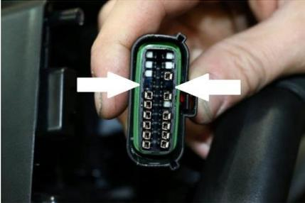
Insert the green connector wire into port 7, insert the yellow connector wire into port 17.
