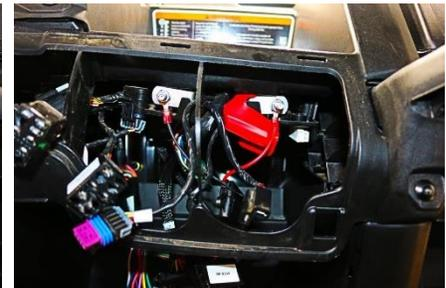
13. Verify operation of all lights. Cable ties any extra harness under dash. Reinstall center tunnel.
