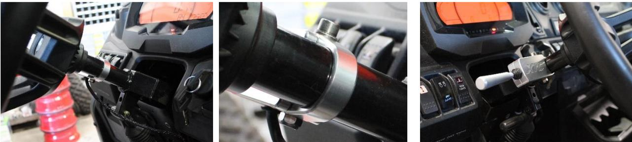
If desired, the plastic cover can be cut and re-installed so that the lever goes through.
