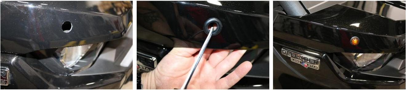
7. **Attach Front Harness to lights** - The Green and white wire go to the right/passenger side LED, attach the Green to the Black and the White to the White, the Yellow and white wire go to the Left/Driver side LED, attach the yellow to the Black and the white to the White. NOTE: Black wire is positive and goes to the Green and Yellow wire, they will not work if reversed. White is ground. Pull any excess wire back under the dash and secure the Harness using the provided cable ties.
