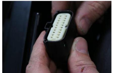
Re-install plastic locking cover, plug connector back into the Instrument Cluster and reinstall assembly.
