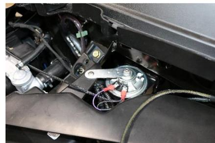
5. **Install Horn** – (shown above right) Using the OEM wire harness clip hole, push it out and mount the horn using the factory hole with the supplied screw and nut. Secure the OEM harness to the horn bracket. Attach Violet and Black wire from front harness to horn terminals, polarity does not matter.
