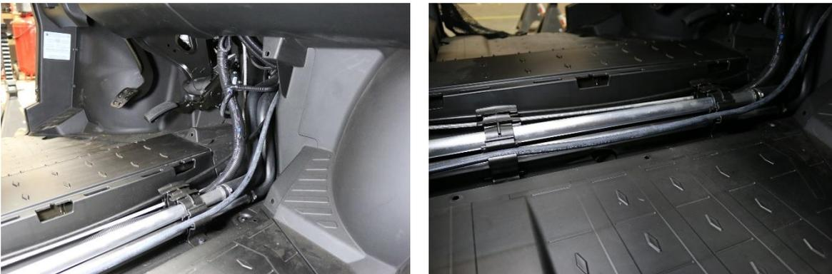
3. **Run the Rear Extension Harness** –Unroll the Long Extension Harness and plug into the new rear harness. Make sure to keep the harness away from any **HOT** or moving parts, run the other side with the 4-pin connector down through the opening that leads into the center tunnel, unlatch the cars cable harness's and insert our harness up to the center dash opening. Secure using the supplied cable ties.
