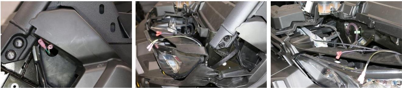
Run the other end with the 4-pin connector to the center cubby where the rear harness was run.
