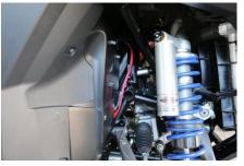
Make sure to run the harness inside of the frame away from the control arm, going through the rubber grommet in the fire wall
