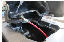
Open the Dash storage and remove the tray, run the harness up into the compartment. Plug into the Control Module. WARNING! Verify that there is clearance where you want to mount the front LED lights before drilling the holes!
