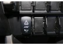
Run Switch Harness—Plug the Switch Harness into the Control Module, run Horn/Hazard connector through the rectangle switch cutout and use included grease on switch terminals then connect Switch and slide into dash. **NOTE:** The switch cut outs are counter sunk, we have supplied 2 switch seals to be used as spacers to keep it raised out of the indent to keep it from getting stuck.
