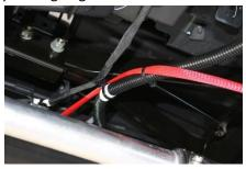
Cross over to the passenger side, secure harness to brake line and battery cable, continue to the front.
