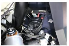
11. Plug the Power Harness into the Control Module. Run the power wire to the Busbar, remove one of the blanks and plug into the Busbar.
