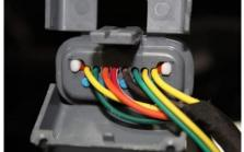
9. Close Cover – Run ATS wires alongside the OEM harness and snap shut, re-install plastic locking cover and plug back in.
