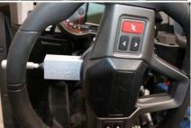
5. Install the Horn/Hazard Switch. Remove 1 of the switch plugs.
