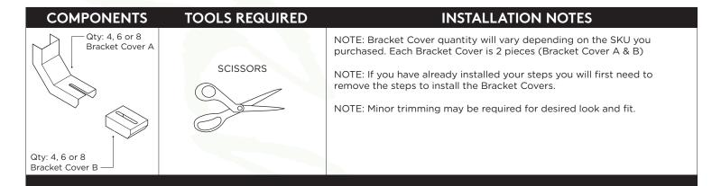
1. Place (1) Bracket Cover A onto the installed bracket to identify if there is any trimming needed.
