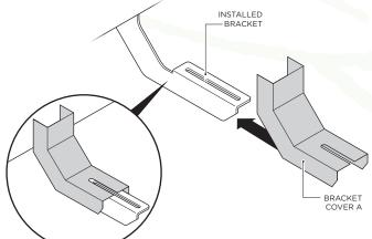
2. If trimming is necessary, carefully trim the Bracket Cover using scissors or a knife until you reach your desired look and fit (2a). Once this is complete, place the Bracket Cover A onto the installed bracket (2b).
