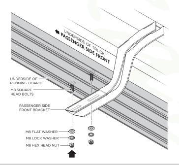
**6.** Fasten the Running Board to the Passenger Side Center Bracket cradle by using (2) M8 Flat Washers, (2) M8 Lock Washers and (2) M8 Nylon Nuts.
