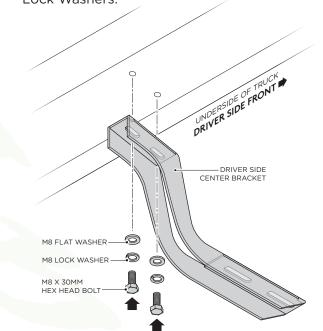
**4.** Fasten the top portion of the Driver Side Rear Bracket by using (2) M8 x 30MM Hex Head Bolts, (2) M8 Flat Washers and (2) M8 Lock Washers.
