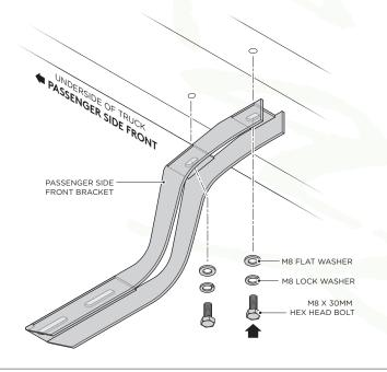
**3.** Fasten the top portion of the Passenger Side Center Bracket by using (2) M8 x 30MM Hex Head Bolts, (2) M8 Flat Washers and (2) M8 Lock Washers.
