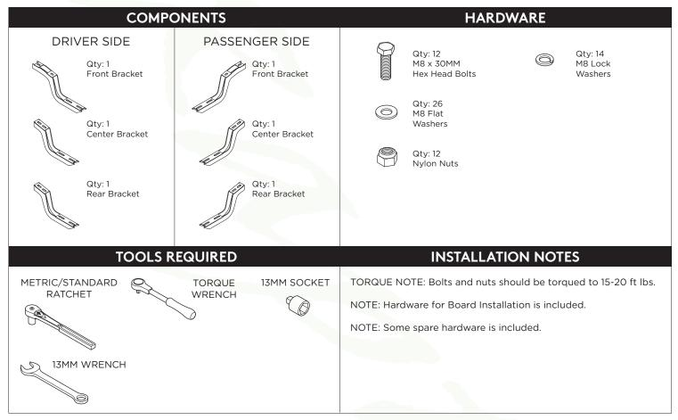
Remove all contents from the package and check brackets for any damage. Also, verify that all components and hardware listed above are included before you begin installation. If anything is missing or damaged please contact us at customerservice@raptorseries.com
