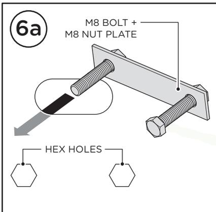
Rotate the threaded side of the M8 Bolt + M8 Nut Plate to the bottom left hole.
