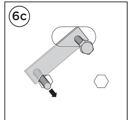
Install Plastic Retainer to ensure you do not drop the M8 Bolt + M8 Nut Plate into the rocker panel.
