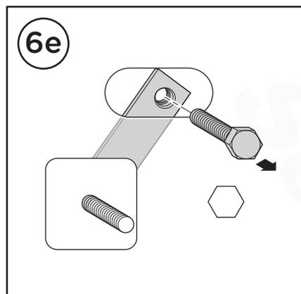
The M8 Nut Plate will now be able to rotate down to the hole in the rocker panel, allowing for bracket installation.
