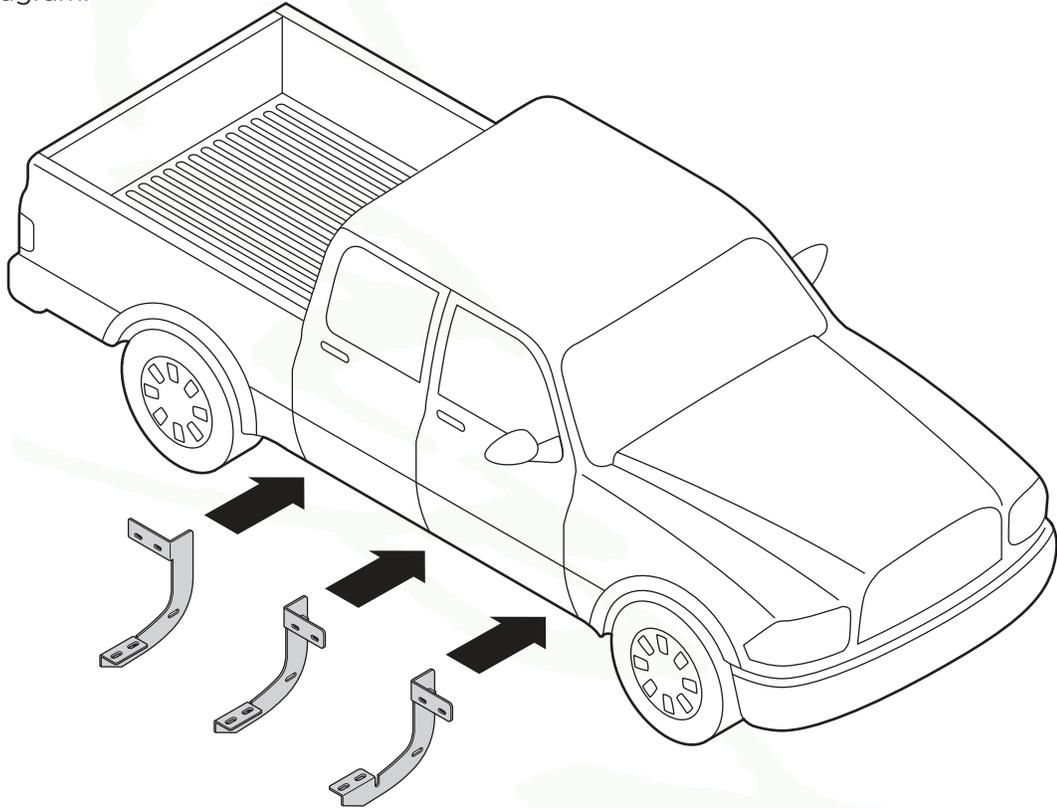
2. Passenger Side Front Bracket cradle (2a) will face to the rear of the truck. Passenger Side Center (2b) and Rear Bracket cradles (2c) will face toward the front of the truck.
