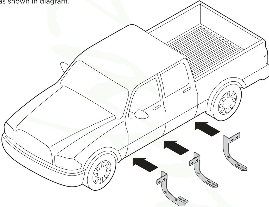
2. Driver Side Front Bracket cradle (2a) will face to the rear of the truck. Driver Side Center (2b) and Rear Bracket cradles (2c) will face toward the front of the truck.
