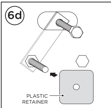
Remove the M8 Bolt from the M8 Nut Plate.
