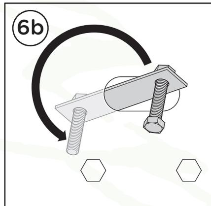
Pull the threaded side of the M8 Bolt + M8 Nut Plate through the bottom left hole.
