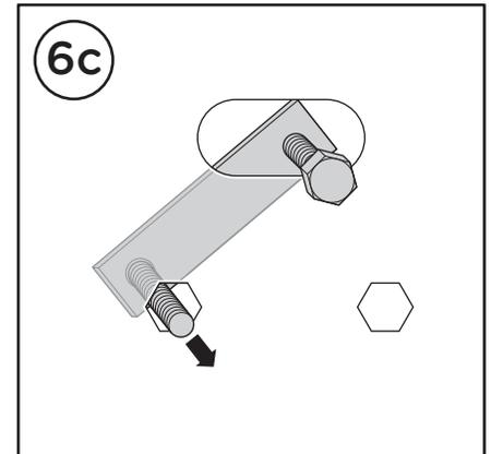
Install Plastic Retainer to ensure you do not drop the M8 Bolt + M8 Nut Plate into the rocker panel.
