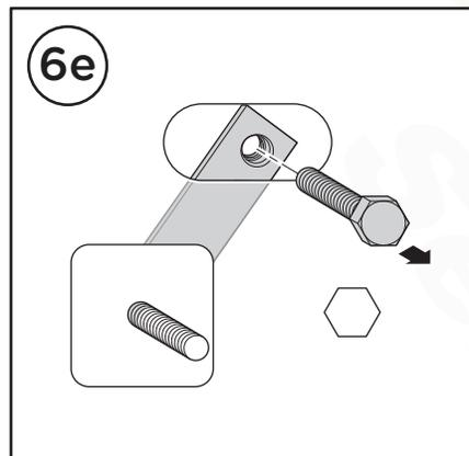
The M8 Nut Plate will now be able to rotate down to the hole in the rocker panel, allowing for bracket installation.
