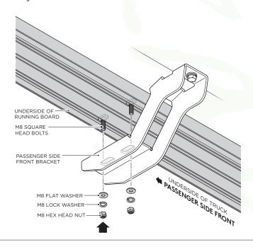
**6.** Fasten the Running Board to the Passenger Side Center Bracket cradle by using (2) M8 Flat Washers, (2) M8 Lock Washers and (2) M8 Nylon Nuts.
