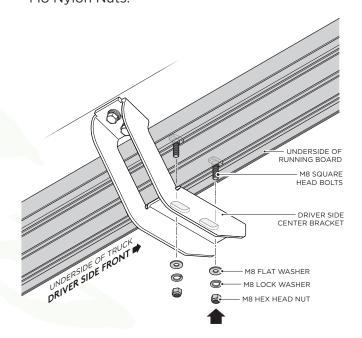
7. Fasten the Running Board to the Driver Side Rear Bracket cradle by using (2) M8 Flat Washers, (2) M8 Lock Washers and (2) M8 Nylon Nuts.
