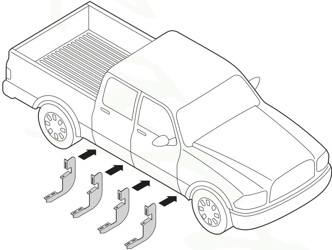
2. Passenger Side Front Bracket cradle (2a), Passenger Side Center Bracket cradles (2b, 2c), and Passenger Side Rear Bracket cradle (2d) will all face towards the front of the truck.
