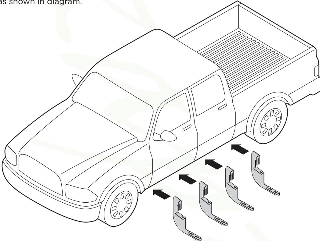
2. Driver Side Front Bracket cradle (2a), Driver Side Center Bracket cradles (2b, 2c), and Driver Side Rear Bracket cradle (2d) will all face towards the front of the truck.
