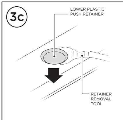
Pull the lower Plastic Push Retainer out of the rocker panel to expose threaded holes that will be used for bracket installation.
