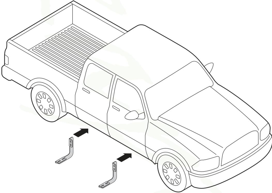
2. Passenger Side Front Bracket cradle (2a) and Passenger Side Rear Bracket cradle (2b) will face toward the front of the truck.
