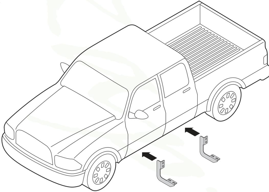
2. Driver Side Front Bracket cradle (2a) and Driver Side Rear Bracket cradle (2b) will face toward the rear of the truck.
