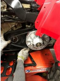
6. Slide belt into DURACLUTCH DCR Primary clutch then install on post. Use stock primary hardware removed in step 4- spacer, washer and lock washer. Tighten bolt to 47 ft-lbf.
