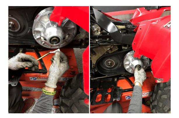
4. Remove Primary clutch bolt. Remove the stock Primary clutch with puller SVI PN# 25-126. Greasing the end of the puller slightly will aid in removal. Do not get grease on any clutch components. Clean the engine tapered shaft and Primary clutch bore with alcohol or degreaser. Do not lubricate.
