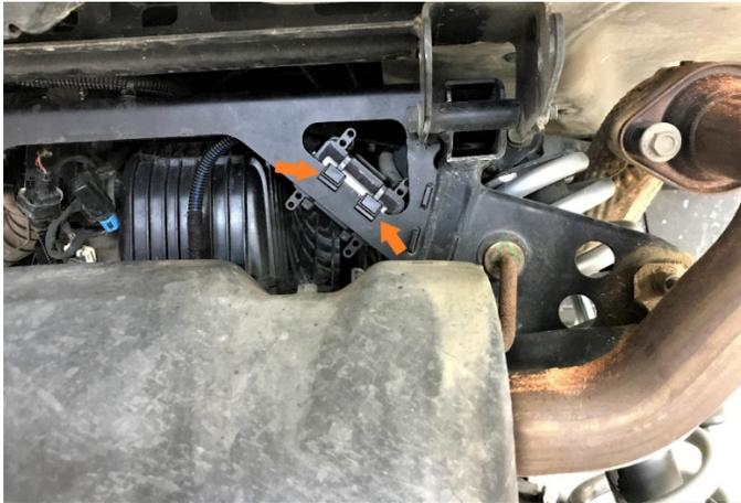
17. Take two 8-inch cable ties and feed thru tab on top of dongle housing and around the frame and tighten
