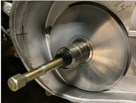
8. Clean the engine tapered shaft and Primary clutch bore with alcohol or degreaser. Do not lubricate.
