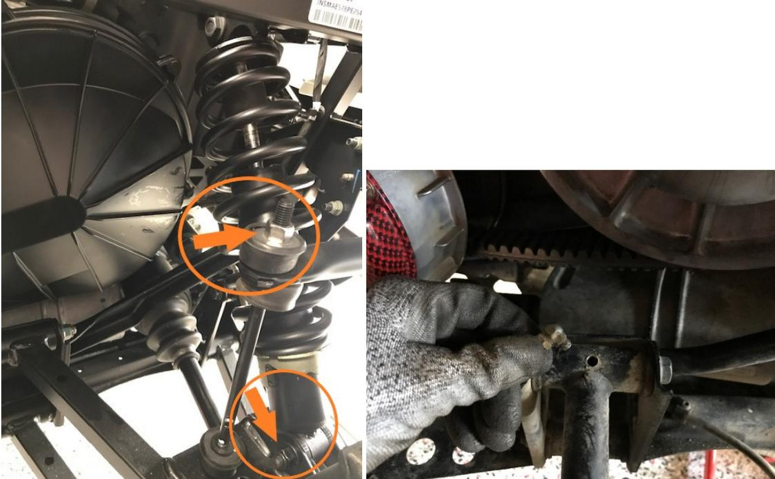
3. Remove stock secondary clutch. Pay attention if there is a snap ring on the shaft and if there are any washers on the shaft with the snap ring. If there is a snap ring or washers remove them. There also may be washers on the spine at the end of the shaft. If there are any remove and discard.
