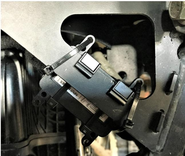
18. Disconnect speed sensor on transmission. Connect end from dongle to transmission. Connect wire removed from transmission into other end of dongle. Make sure Dongle does not interfere with any moving components, such as suspension or shifting assembly. Use remaining cable ties to secure wires as necessary and clip excess tie ends.
