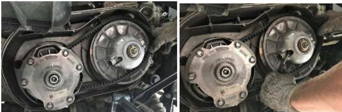
9. Once primary is torqued, with transmission in PARK, spin secondary clutch back & forth a few times to allow belt back to top of secondary.
