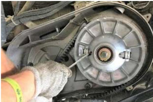
6. Slide belt into primary clutch, then install on post.
