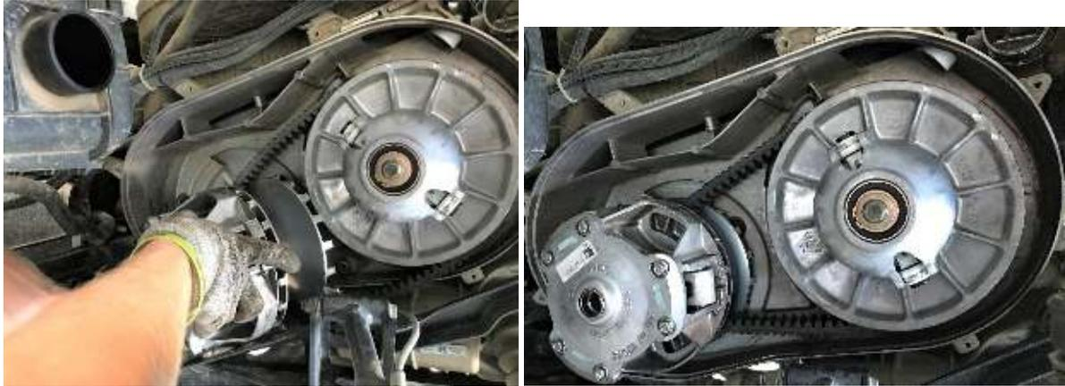
7. Install DURACLUTCH Primary with shoulder washer as shown. DO NOT USE the O.E. flat washer or lock washer. The flat washer will interfere with the primary cover. Tighten bolt to **60 ft-lbs. VERY IMPORTANT-** Over tightening will not allow clutch to operate properly and cause damage and failure of the clutch.
