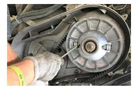
9. Slide belt into primary clutch, then install on post.
