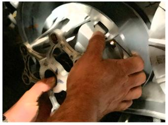
4. Pull the Polaris primary fixed sheave from the engine crankshaft using PN 99-012 puller. Greasing the end of the puller slightly will aid in removal. Do not get grease on any clutch components.
