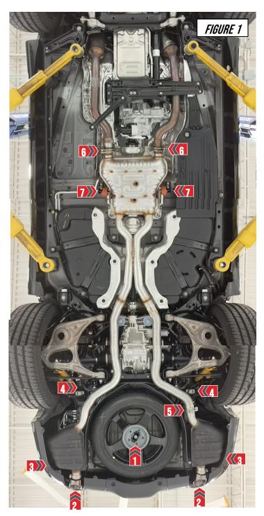
Start by removing the OEM Durango exhaust by following these steps, shown in **Figure 1**.
