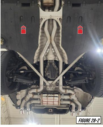
Fully tighten down all four clamps, and ensure that nothing has moved or is contacting the chassis or bracing anywhere.
