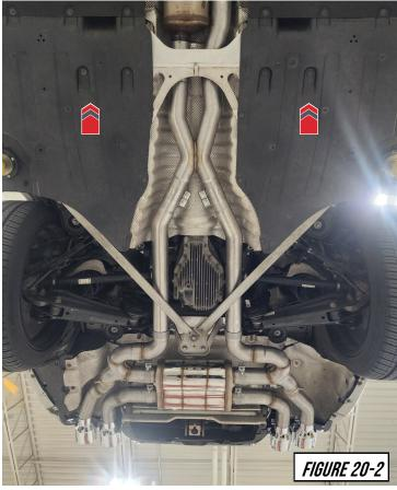
Make your final adjustments to the tips to ensure they are in a position you like. Once the desired positioning is achieved work from the front of the car to the back, tightening all the clamps fully and ensuring there is proper clearance of the chassis, and braces.
