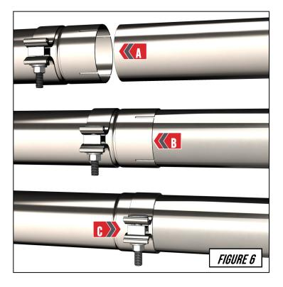
Install your AWE passenger side axle tube (**G94**) as shown in **Figure 7-1**. Secure a provided lock collar flush on the end of the hanger bar then reinstall the OE hanger as shown at (**A**). Next slide the inlet side of the tube into the sleeve clamp (**B**), and snug the clamp but do not fully tighten it at this time.
