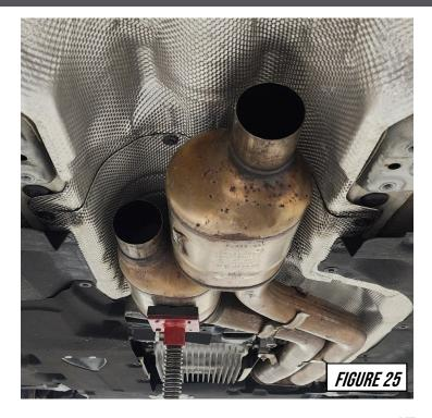
It is crucial to install each section and exhaust band clamps correctly to prevent loose joints. exhaust leaks and rattles.
