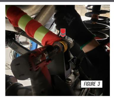
Remove the OE tip sections from the driver and passenger side of the vehicle, as shown in Figure 4.
