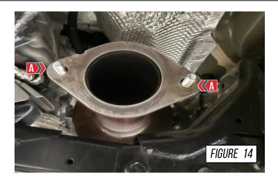
Now install your AWE inlet sections, making sure that the tooth (A) on the flanges of both pipes are facing down from the body of the truck.
