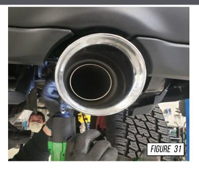
To install the exhaust tips with integrated clamps, first, attach the exhaust tip in the proper orientation onto the exhaust outlet tube.
