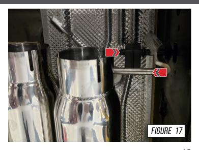
Once the H-pipe is in proper position, tighten the two clamps at the inlet of the H-pipe then tighten the bolts on the inlet flanges.
