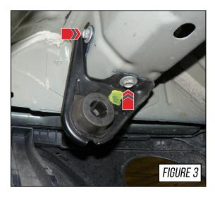
Transfer the hanger bushing and bracket assemblies from the OEM exhaust to the correlating AWE components.
