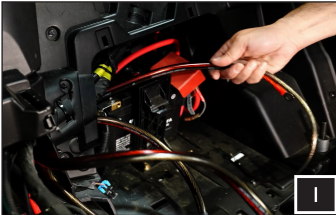
I. Route the power cables along the driver side center console from the battery location towards the driver side dash.
