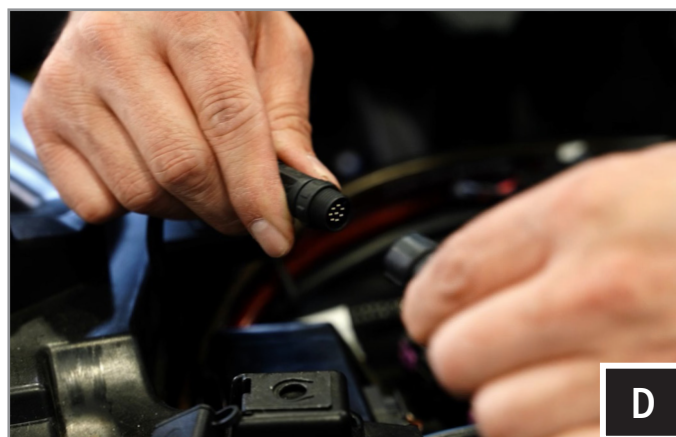
D. Plug in the LIT-CC controller to the LIT-CC module.
