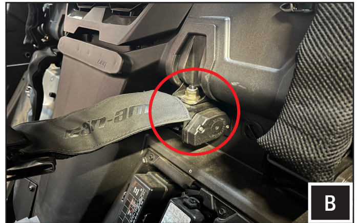
B. Start the install by removing the driver seat. Use an 18mm socket wrench to remove the right shoulder seat belt retractor mechanism.
