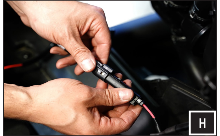
H. Plug in the subwoofer connector to the Y splitter.
