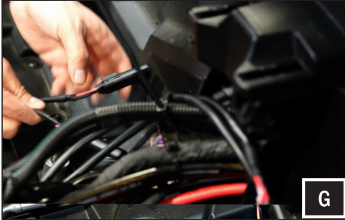
G. Use the provided B-H3081 audio “Y” splitter to power the 2 subwoofers.
