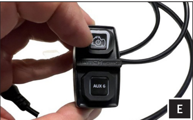
E. Select the icon inserts and press in the icon insert into the silicone push button membrane. Note that button one is on top when reading the SWITCHWORKS logo on the controller. This is important when programming for settings.
