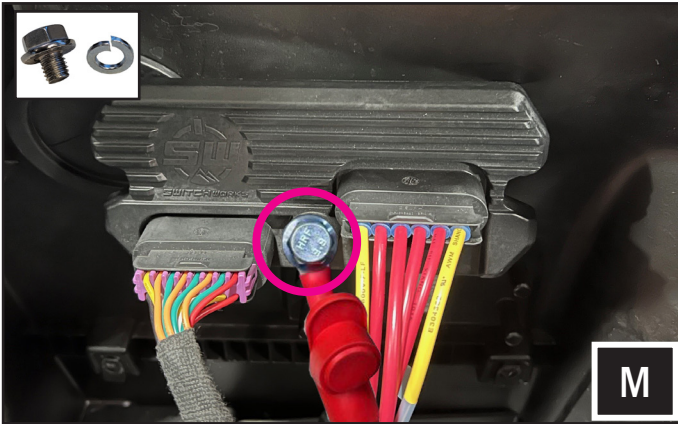
M. Connect the main power cable to the RS6 Switcher module using the provided M8 bolt and split washer.
