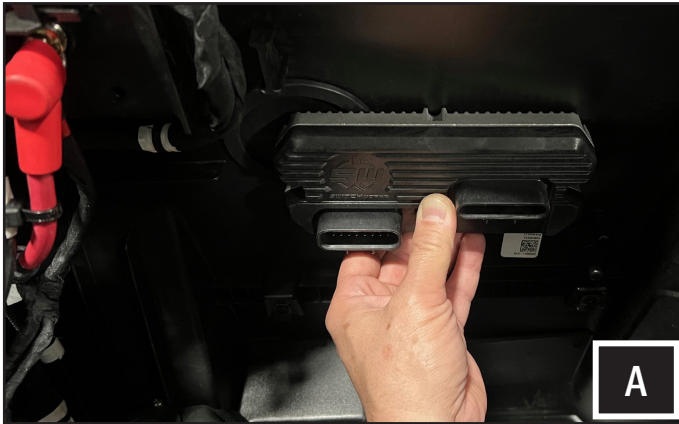
A. Mount the RS6 Switcher module on the firewall or a panel in the vehicle where it can be accessible to plug in harnesses.
