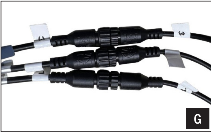
G. Plug in the RS6 Switcher controllers to the matching connectors on the Power and Switch harness (B-H3013).
