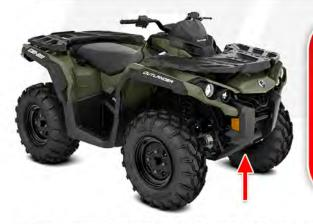
PLACE JACK UNDER THE CENTER OF FRONT AND LIFT UNTIL THE WHEELS ARE OFF THE GROUND. BE CAREFUL TO SECURE PROPERLY SO IT IS STABLE ON THE JACK OR JACK STANDS. REMOVE TIRES.
