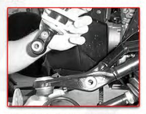
NOW, REMOVE THE COTTER PIN FROM THE UNDERSIDE OF THE TIE ROD AT THE KNUCKLE AND THEN DISCONNECT THE TIE ROD(14MM SOCKET). NOW REMOVE THE UPPER CONTROL ARM FROM THE FRAME AND KNUCKLE USING A 15MM SOCKET.
