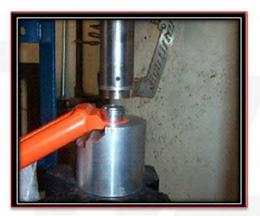
4. WHEN PRESSING THE BALL JOINT, BE SURE TO FULLY SEAT THE BALL JOINT SO THE SNAP RING CAN BE FULLY SEATED. MAKE SURE TO CLEAN THE SNAP RING GROVE OF ANY PAINT OR MATERIAL THAT MAY HAVE BECOME LODGED IN THE GROOVE DURING THE PRESS OPERATION. WE RECOMMEND YOU USE A PICK OR FINE POINT TO CLEAR THE SNAP RING GROOVE. USE A SNAP RING TOOL TO SECURE THE SNAP RING INTO PLACE.
