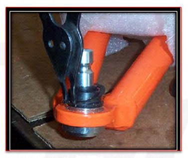
NOTE: IF THE BALL JOINT IS PRESSED IN TOO HARD IT WILL CRACK THE PAINT. IF THIS HAPPENS THEN TOUCH UP PAINT CAN BE APPLIED.
