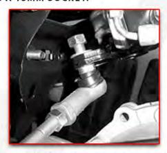
NEXT, REMOVE THE LOWER INNER BOLTS FROM THE FRAME ON THE LOWER CONTROL ARM THEN REMOVE THE LOWER ARM FROM THE KNUCKLE ASSEMBLY USING A 15MM SOCKET.
