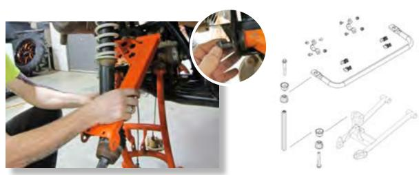
Remove the lower shock bolt connected to the lower control arm. Remove the upper arm first by removing the bolts at the frame then disconnect the lower arm at the frame.
