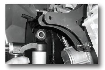
Connect the top of the shock to bracket using a 10x65mm bolt (MCS10X65-10.9) and lock nut (MLN10-1.5). Connect the bottom of the shock to the control arm using a 10x65mm bolt (MCS10X65-10.9) & lock nut (MLN10-1.5).
