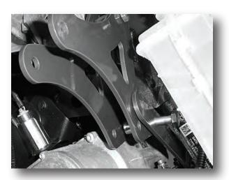
Between the two brackets, insert a (CCC spacer) and the second cross bracket.
