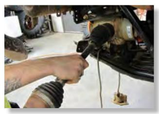
Remove the stock axle from the rear differential.
