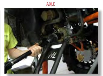
Use the factory hardware to connect the new lower arm to the frame. (18mm) Then Insert the axle into the differential.
