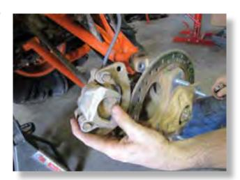
Remove the brake caliper mounting bolts (15mm)
