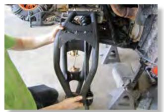
Install the upper control arm at the frame, secure it with the factory hardware.
