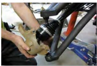
Insert the axle into the knuckle then the lower ball joint, secure it insert the bolt. (13mm)
