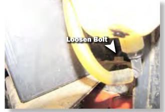
You will have to remove the bolts attaching the battery mount plate to the frame to access the frame bolts on the upper arms (13mm). Loosen the bolts on the plate that connect to the bumper; this will help move the plate out of the way. YOU DO NOT HAVE TO REMOVE IT. MOVE OVERFLOW RESERVOIR OUT OF THE WAY TO ACCESS BOLT.
