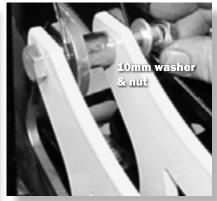
Slide a 10x65mm bolt (MCS10X65-10.9) through the lift bracket (35Q) followed by a 10mm washer (MFW10). Place the bracket to the outside of the rear shock mount tab (from the rear). Place a (NNN spacer) between the factory shock mount tabs and lift brackets. Install the other (35Q) lift bracket to the inside of the shock tab. Install a 10mm washer, then loosely secure the bolt with a 10mm lock nut (MLN10-1.5).
