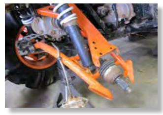
Remove the upper and lower bolts connected to the knuckle assembly. KEEP ALL FACTORY HARDWARE.
