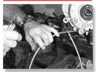
Connect the provided T-block to the new (37X) brake lines to the block. Once the lines are both connected, Secure it to the frame using the factory hardware. Route the lines down to their corresponding hubs.
