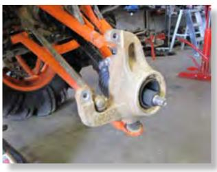
Remove the cotter pin, axle nut, and washers from the hub assembly, then remove the hub. (27mm)
