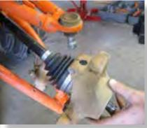
Disconnect the Upper ball joint by removing the bolt at the knuckle.
