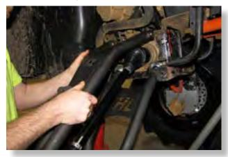
Install the new upper control arm to the frame and secure it with factory hardware.
