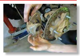
Connect the caliper to the hub assembly by using the (2) 10x25 button head bolts.
