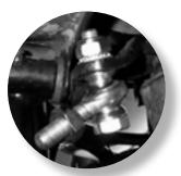
Lightly dab loctite onto the bolt and secure it tight with the 10mm lock nut (MLN10-1.25).
