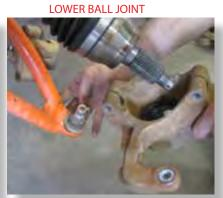
Disconnect the Lower ball joint by removing the bolt at the knuckle. (13mm)
