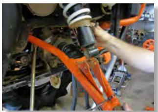
Remove the Upper and Lower arms by removing the bolts from the frame and the bolts from the shock on the upper arm. Completely remove the shock. (18mm) KEEP ALL FACTORY HARDWARE.
