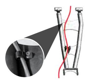
Route the brake line through the shock tabs on the lower arm. Secure it in place using a p-clamp and 5x16mm bolt followed by a 5mm washer and 5mm lock nut.
