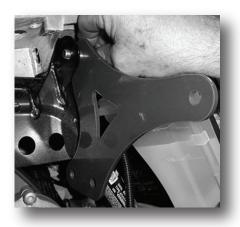
Between the two factory shock mounting tabs place the (CCC spacer) and second bracket. Now slide the bolt through the shock mount, spacer, and bracket.
