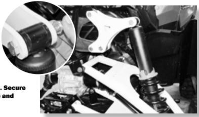
Attach the shock to the upper lift bracket. Secure it using a 10x65mm bolt (MCS10X65-10.9) and 10mm lock nut (MLN10-1.5).
