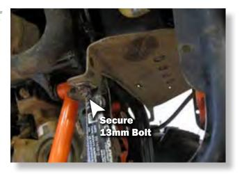
Re-secure the bolts that were previously loosened and removed from the battery mount bracket. (13mm). RE-SECURE OVERFLOW RESERVOIR.
