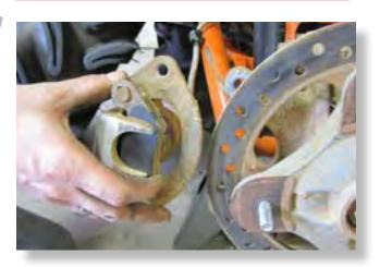
**Disconnect the caliper** bolts from the hub assembly, leave the brake line attached to the caliper (15mm). Set brake caliper aside. **KEEP FACTORY HARDWARE**.
