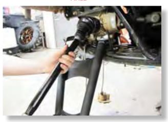
Install the new adjustable lower arm, secure at the frame with factory hardware. Install the axle into the differential.
