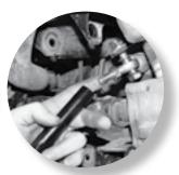
Secure the inner tie rod to the heim by threading it onto the heim joint.
