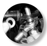
Now connect the heim joint to the steering stem. Insert the bolt up from the bottom. Next place a flat 10mm washer (MFW10), and a 10mm lock washer (MLW10Z) on the bolt.
