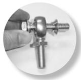
Using a 10mmx50mm bolt, place a Hi-misalignment cone (43Z) on each side of the heim joint.
