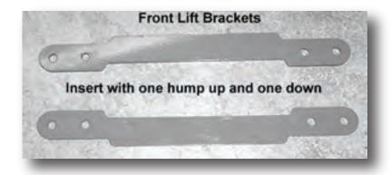
Now insert the cross bracket into the frame and slide the bracket across the opposite side. The cross bracket will go on the outside of the front lift bracket. You need to install the brackets so that the bracket that is to the front of the ATV has the hump in the downward position and the bracket closest to the power steering unit has the hump in the upward position.
