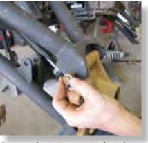
Connect the **hub assembly** by using the **stock bolt** to secure the **upper control arm.**
