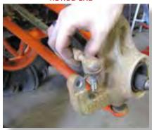
Disconnect the tie rod by removing the cotter pin, nut, and washer from the knuckle. (15mm)
