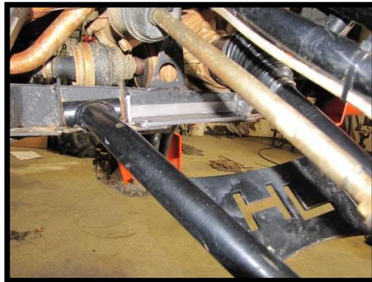
8. Next connect the left and right rear bracket to the control arm tabs. Place a 10mm flat washer on the 10mm x 110mm bolt. Insert the bolt through the brackets and control arm collar. Loosely secure the bolt and brackets with a 10mm washer and 10mm lock nut.
