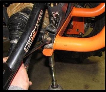
5. Once you have removed the bolts it is time to connect the frame plate brackets. There are left and right brackets. For orientation, left and right is determined from the seated position. Images used in for instructions are from the right side.
