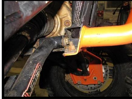
4. If you have a bumper, remove the two bolts that connect the lower portion of the bumper to the frame. These are located near the lower control arms.
