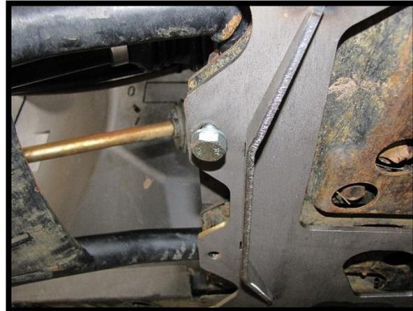
12. On the top side of the frame rail, loosely connect the plate with a 10mm washer and 10mm lock nut. Repeat steps until all bolts are in place.
