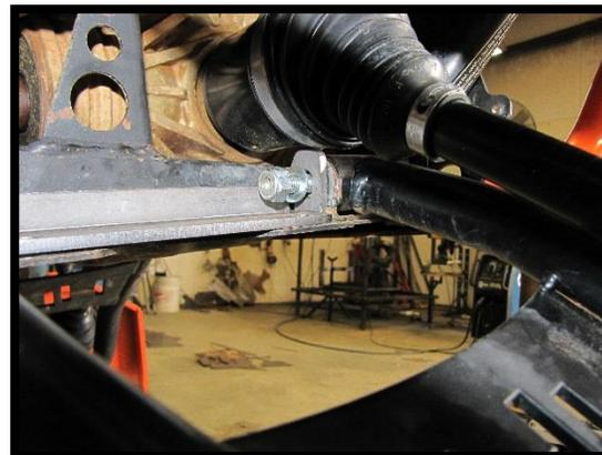
10. For the second stage, connect the frame support plate to the under carriage of the UTV. The rib side of the place faces outward, the flat side faces the frame.
