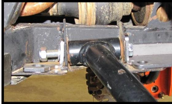
9. Next connect the front left and right bracket to the control arm tabs. Place a 10mm flat washer on the 10mm x 110mm bolt. Insert the bolt through the brackets and control arm collar. Loosely secure the bolt and brackets with a 10mm washer and 10mm lock nut.
