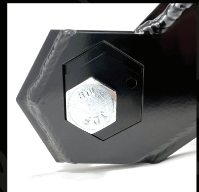
Highest caster setting +4° (5"-6" Lift with no drop bracket)
