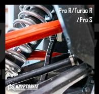
The hex shaped ends should be the 'top' of the end link when installed.
