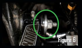
**6**. Grab your new Kryptonite upper control arm ensuring the logo plate is closest to the front of the truck. Install the hardware including the washers on the outside of the of the bushings. The ball joint will be mounted on the top side of the control arm. The control arm bolts will be torqued to (89ft/lbs + 45°)
