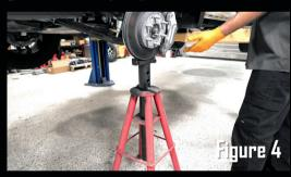
4. Loosen the upper control arm hardware slightly to lift the OEM arm out of the way. You will now address the final nut on the top of the strut, allowing you to completely remove it from the vehicle.
