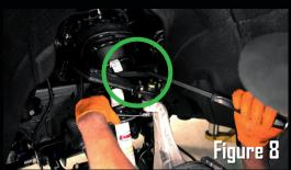
8. With the strut in place you will remove the nut from the upper ball joint stud and seat the taper into the knuckle. You can apply downward pressure to the upper control arm with a cushion (rubber pad - Figure 8) or using a 6mm allen to hold the stud while tightening the nut with an 18mm wrench. Figure 9 - This nut will we torqued to the DEM spec (26ft/lbs + 60°) to seat the taper.
