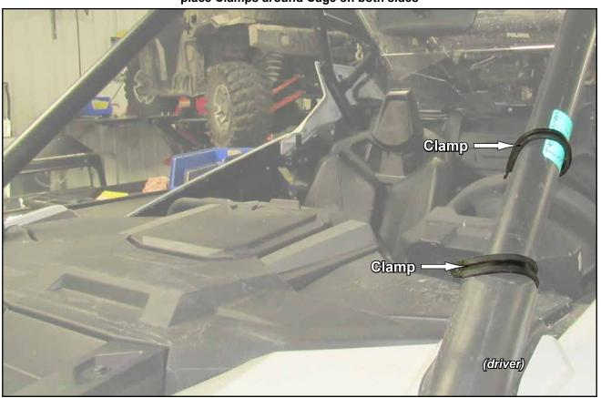
place Windshield onto machine and secure to Clamps with previously removed Clamp hardware
