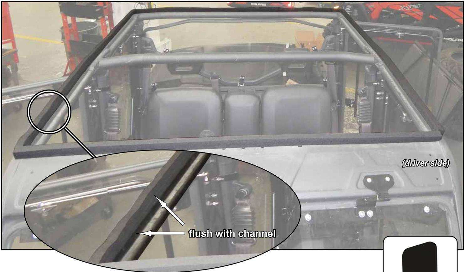
**Install Brackets and Foam only if SuperATV Rear Windshield is installed.**
