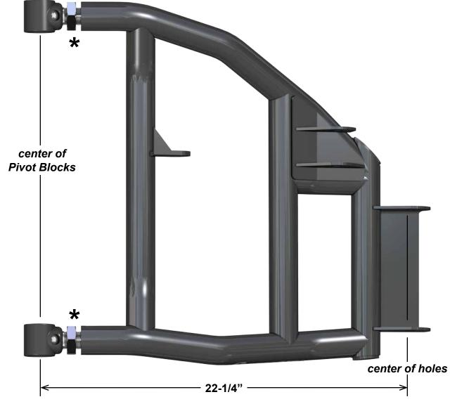
\*Leave Jam Nuts loose. Tighten after final adjustments have been made.
