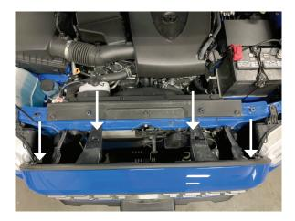
**Step 2:** To release the grill, pull the grill directly away from the front of the vehicle. Once the grill is removed, place it in a safe location. Locate the plastic retainer clip on the plastic splash guards. Remove the retainer clip and then remove the splash guard on each side.
