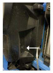
**Step 3:** Locate the factory frame bolts on the outside edge of the frame rails. These bolts will need to be removed. To remove the bolts use a 14mm socket wrench. They are usually very tight, therefore we recommend using a tool with a long handle.
