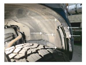
**Step 2:** Locate one "push-in" style plastic retaining clip, and with a flat head screwdriver, remove the top piece of the clip. Once removed, remove the bottom part. Several pressure clips hold on the trim piece. Working your way from the top to the bottom and then to the exterior to remove the piece. Do not remove the trim piece all of the way. Continue to step 3.
