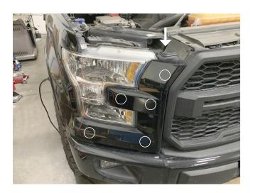
**Step 3:** The two clips shown in the picture are designed not to be removable and are very difficult to workaround. The clips can remove them by squeezing the flared end of the pins with a pair of pliers and pushing them back through the hole. If that method is unsuccessful, the clips can be removed from the fender flair by sliding one clip up and one clip down. The main goal of this step is to get the trim piece entirely removed to gain access to a set of 10mm bolts.
