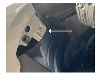
**Step 2:** Pull the inner fender liner away from the bumper and hold it to the side. This will allow you to see the rear side of the factory fog light. The factory fog light is held in with one Philips head screw located on the light's top exterior side. Remove the screw, unplug the light, and place it in a safe location. Take note of how the light is held in our Quattro will mount the same way.
