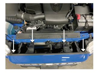
**Step 2:** To release the grille, pull the grille directly away from the front of the vehicle. Once the grill is removed, place it in a safe location. Locate the plastic retainer clip on the plastic splash guards. Remove the retainer clip and then remove the splash guard on each side. The factory fog light should now be visible.
