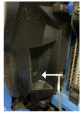
**Step 3:** The factory fog light is held in with one Philips head screw located on the light's top exterior side. Remove the screw, unplug the light and place it in a safe location. Take note of how the light is held in our Quattro will mount the same way.
